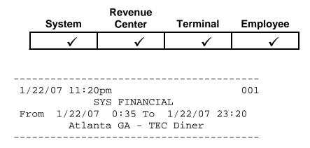
**Readings -** Non-resettable totals maintained by each POS Terminal. This section prints if the USE NRGT option in System Setup is set. These fields do not appear on the Employee Financial Report.
